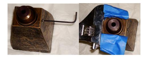
6. Apply Teflon tape to the threads on the ball joint. Using a 1/4" Allen wrench (not provided), thread the ball joint into the shower arm until secure.
